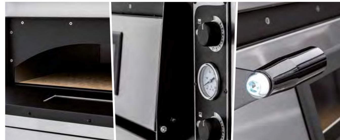
**The electric oven is made of stainless steel and prepainted steel and it is equipped with:** cooking surface in refractory stones, 3 Sheathed heating elements on the top and 3 on the bottom, removable glass door for a better cleaning, internal lighting, rock wool insulation. The design is enriched by a little hood, which makes the oven elegant. The standard power supply is 400 Volt three phases + neutral. Special Voltages are available on request.
